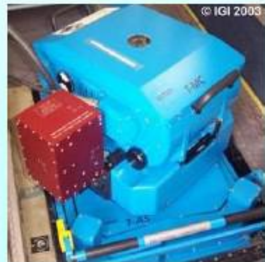
© IGI 2003 System installation AEROcontrol test IMU-Iid mounted at RMK-Top camera
