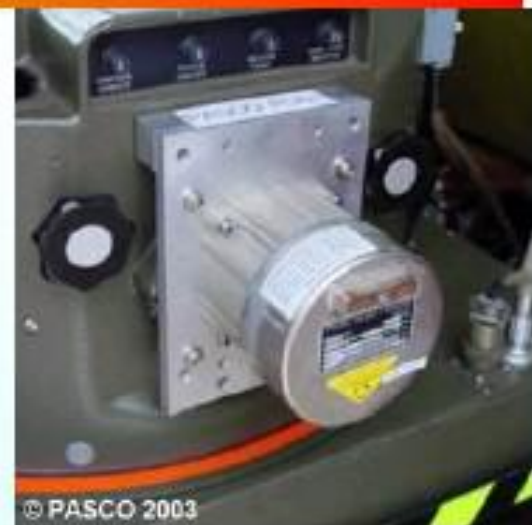
© PASCO 2003 System installation POS/AV test LN200 IMU mounted at RC30 camera
